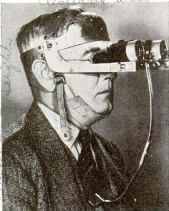
Resting on the platform extending from metal headgear, the field glasses are held steady at eye level
